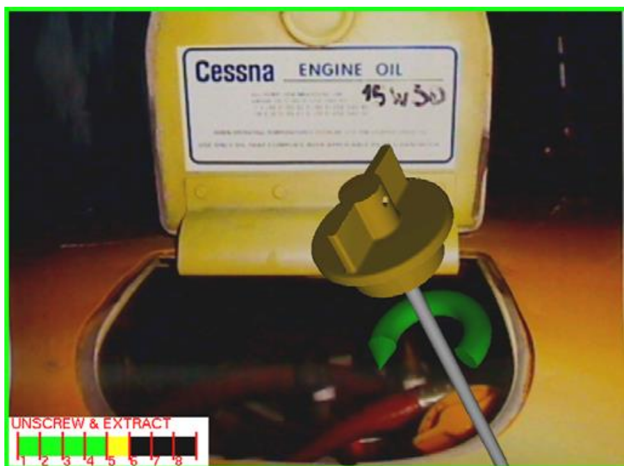
FIGURE 16 THE VIRTUAL LAYER OVERLAID ON THE VIDEO STREAM (ABOVE: STEP 4; BELOW: STEP 5)
